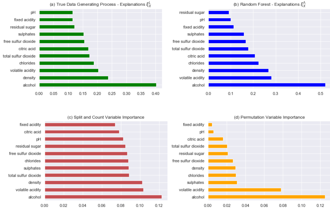
Figure 2.2: Panel 2.2a: dataset explanations \hat{\xi}_i^L based on the 1-norm separation. Panel 2.2b: prediction explanations \hat{\xi}_i^A based on the 1-norm separation. Panel 2.2c: Split and Count measure \widehat{SC}_i , Panel 2.2d: Permutation Importance measure \widehat{PI}_i , for i = 1, \dots, n_X — tabular data.
