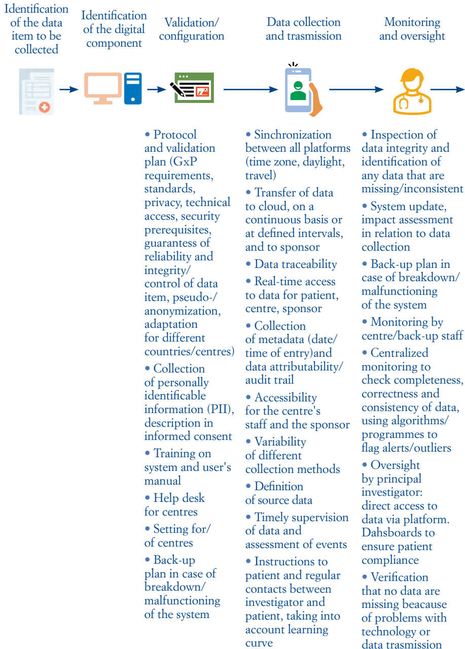
Figure 4b - Data flow diagram - Digital component
