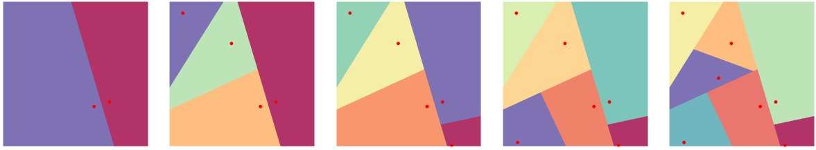
Figure 3.5: Hierarchical Voronoi tessellation of a tensor of size D = 2 , corresponding to \mathcal{L}_j for j = 1, \dots, 5 . Centers are sequentially added and previously-identified areas are further divided into smaller pieces. The step-wise construction implies that only the first plot on the left is a Voronoi tessellation of the 2D surface.
